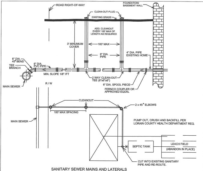
ALL SANITARY SEWERS, LATERALS AND FITTINGS SHALL BE MADE OF POLYVINYL CHLORIDE (PVC) MANUFACTURED TO MEET ASTM SPECIFICATIONS D-3034-SDR 35.
