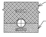
BACKFILL SHALL BE FREE FROM DISCARDED CONSTRUCTION MATERIAL AND DEBRIS. LOOSE EARTH FREE FROM ROCKS, BROKEN CONCRETE AND FROZEN CHUNKS SHALL BE PLACED IN THE TRENCH IN 6-INCH LAYERS AND TAMPED IN PLACE UNTIL THE CROWN OF THE PIPE IS COVERED BY 12-INCHES OF TAMPED EARTH.
